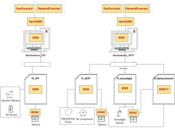
Fig. 4. Hardware-software view w.r.t to the WTP, STP and Streetlight controller
