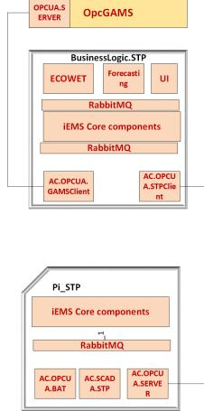
Fig. 5. Software Applications communicating with each other at STP
