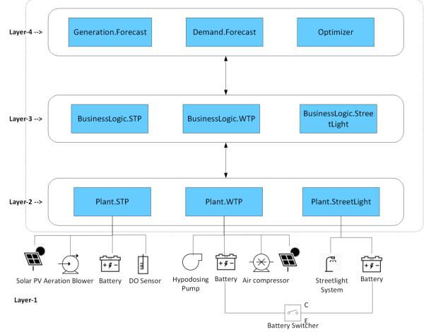
Fig. 1. System Architecture: Hardware-Software view
