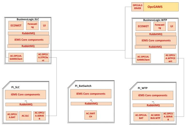
Fig. 6. Software Applications communicating with each other at WTP
